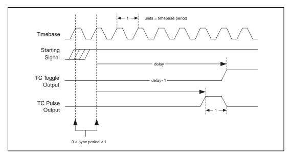
Figure 2-10. Pulse Timing for pulseWidth = 0
